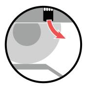
Remove the oil cap and the oil filter.
