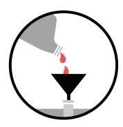
Add new oil using funnel. It is best to place slightly less than the recommended amount.
