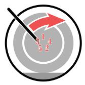
Tighten lug nuts with tire iron in a star pattern.
