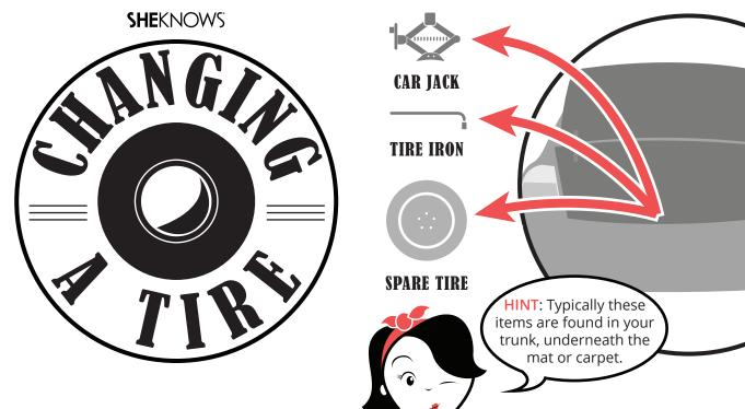
Your car is made with four jack points. The front two are located behind the front tires and the back are in front of the back tires. Find the jack point necessary for your particular tire that needs replacement.
