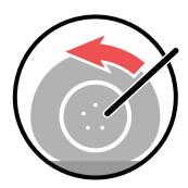
Prior to raising the car, loosen each lug nut with the tire iron. Do not remove, just loosen.
