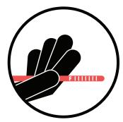
Remove dipstick again and check the fluid's level with the markings on the dipstick.
