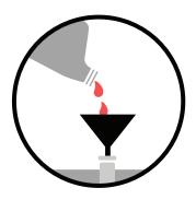
Top off fluid amount, or if low, fill to max. fill line marked on the reservoir.
