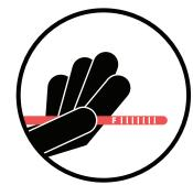
Remove dipstick again and check the oil's level with the markings on the dipstick.
