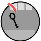
Replace dipstick by pushing it down into position.
